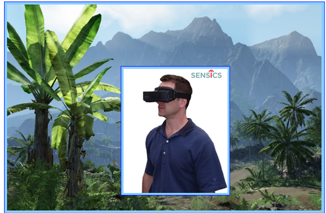
Figure 1: Using an HMD and motion trackers, players will be able to literally walk into this 3D scene, with 360° viewing. Image credits: Crytek GmbH (Crysis game), Sensics Inc (xSight HMD).
