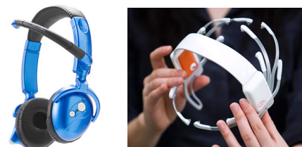
Figure 2: Brain Computer Interface headsets: MindSet by NeuroSky (left), EPOC Neuroheadset by Emotiv Systems (right).
